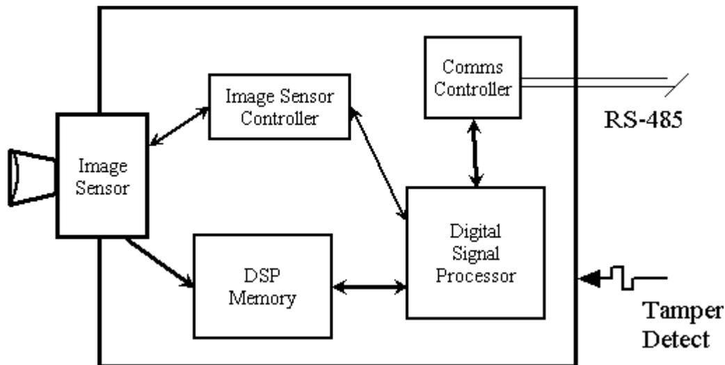
Figure 2: CardaxFT digital camera architecture.
